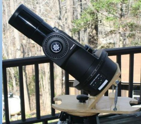
An Alt/Az mount – or an equatorial mount that has not been set up – require the user to move the scope in two rotational axes to follow any observed celestial object.
