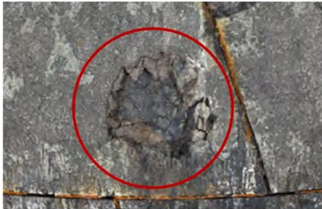
Figure 3: Orion Heat Shield Char Loss After Artemis I Mission
